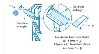
8b Rotate blade and attach (Off-Standard Height Only)
