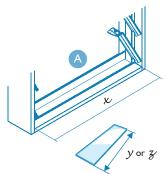
Clips to suit 6mm thick blades . & – 52mm = y Clips to suit 14mm thick blades  $\mathcal{V}$  – 72mm =  $\mathcal{Z}$
